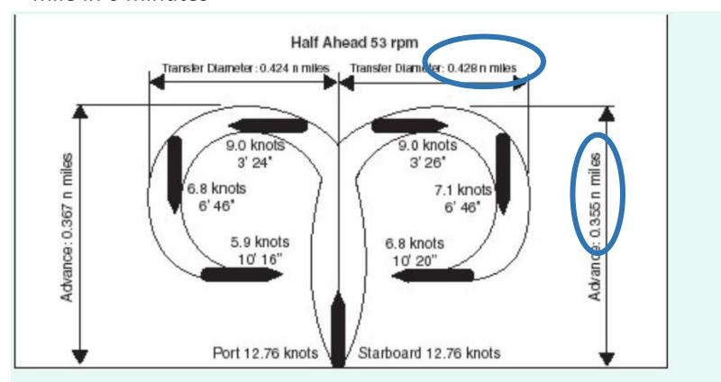
Turning circle - Loaded condition with maximum rudder angle half ahead RPM
